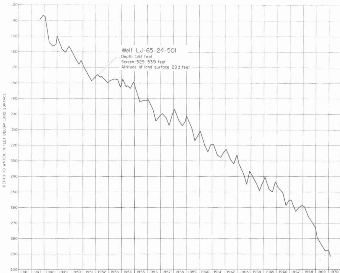
Figure 12.—Changes in Water Levels in a Well Completed in the Alta Loma Sand in the Baytown-La Porte Area
