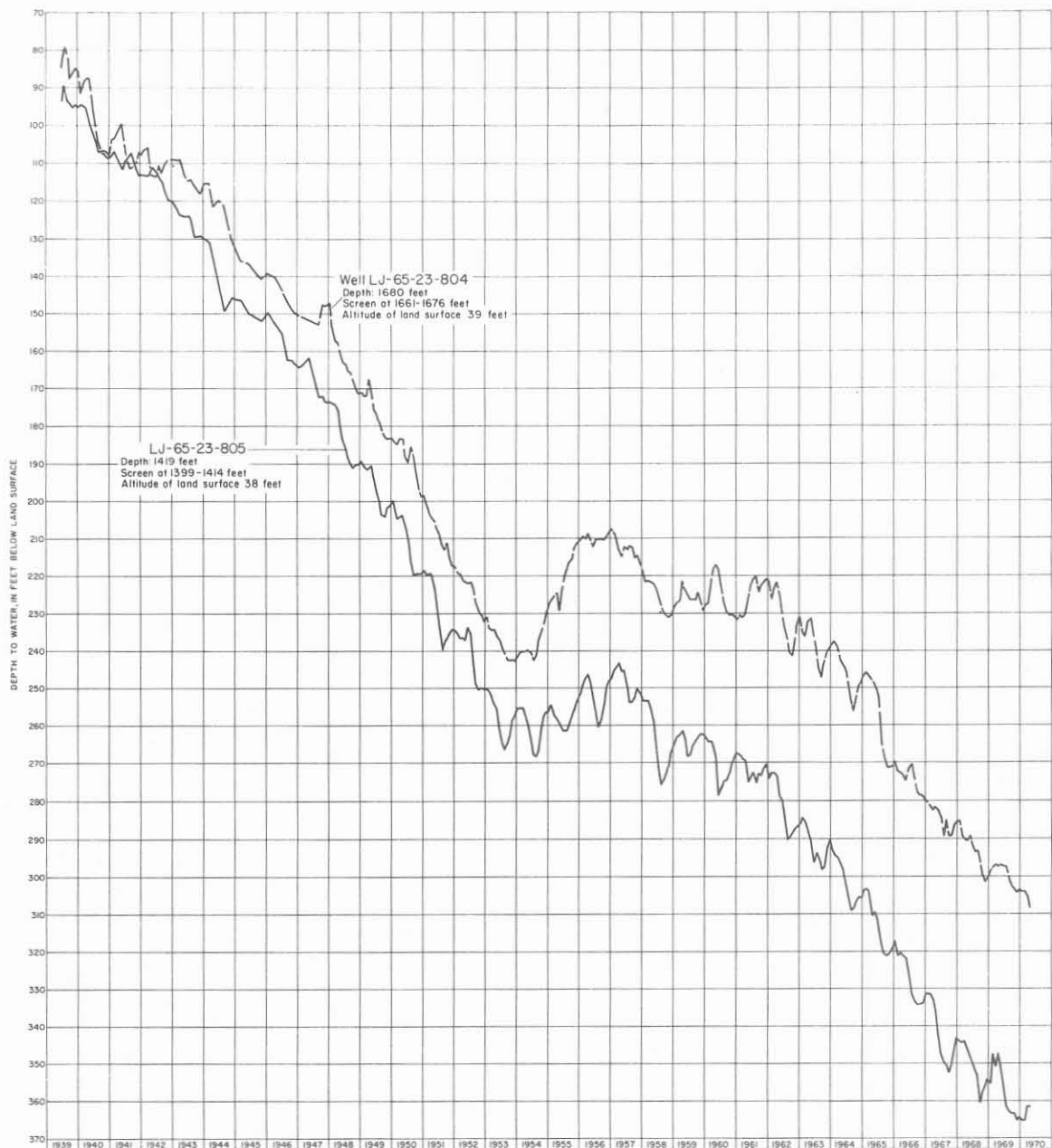
Figure 9.—Changes in Water Levels in Two Single-Screened Deep Wells in the Southern Part of the Pasadena Area
