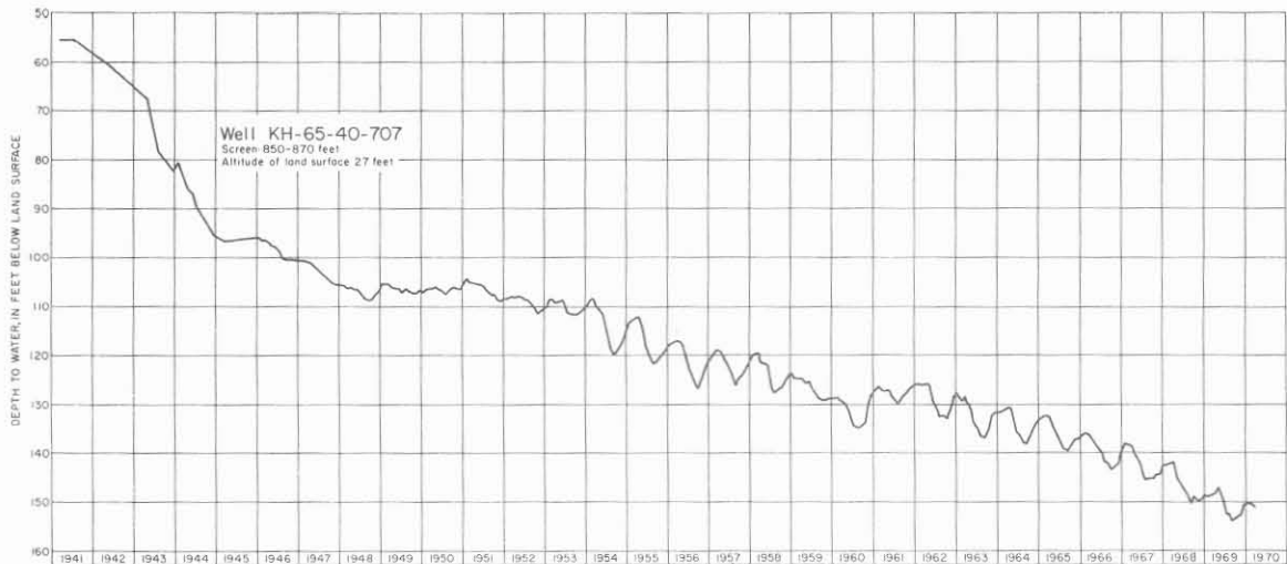
Figure 15.—Changes in Water Levels in Well KH-65-40-707 in the Alta Loma Area
